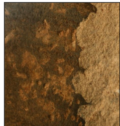
Figure 3c: Deposits along the inner break edge
